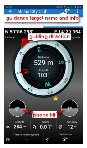
Tapping the tilting indicators opens a menu offering sensor calibration.
