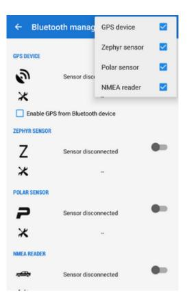
Locus Map can communicate with various Bluetooth-connected external devices - external GPS units, heart rate monitors, bicycle speed&cadence sensors, Zephyr sensors, Polar sensors and NMEA readers. Bluetooth manager displays their switches and settings.
