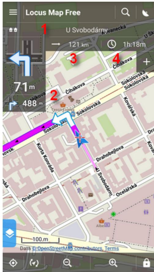
Consists of the **street name/road number indicator** (1), indicator of the **shape and distance of the next two turns** (arrow box)(2) and two **adjustable fields** (3,4) that can display:
