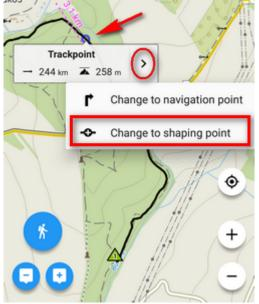
Trackpoint changes into a shaping point and a **new auxiliary point creates in between**:
