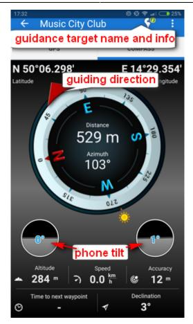
Tapping the tilting indicators opens a menu offering sensor calibration.
