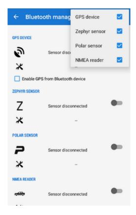
Locus Map can communicate with various Bluetooth-connected external devices - external GPS units, heart rate monitors, bicycle speed&cadence sensors, Zephyr sensors, Polar sensors and NMEA readers. Bluetooth manager displays their switches and settings.
