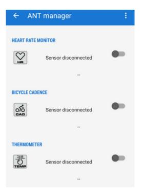
ANT+ is a wireless technology of monitoring devices mutual communication. Locus Map can communicate this way with heart rate monitors, bicycle speed/cadence sensors, stride sensors and many others. More about ANT+ and supported devices here >>
