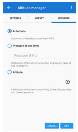
Some devices are equipped with barometric pressure sensor. Barometric sensors measure atmospheric pressure very precisely which can be used for calculating relative altitude changes. I.e. if you know certain pressure at certain altitude you can calculate altitude changes between known and current position.
