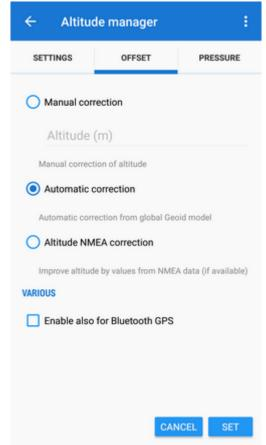
Altitude calculated by internal or external (Bluetooth) GPS unit is related to a different method of referencing the Earth surface than that used in maps. The difference between them is called **Geoid height** which is distance between **Geoid** and reference elipsoid.
