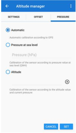
The pressure sensor must be calibrated to a known altitude value so that it can be used for real altitude value calculations. Locus Map offers several methods:
