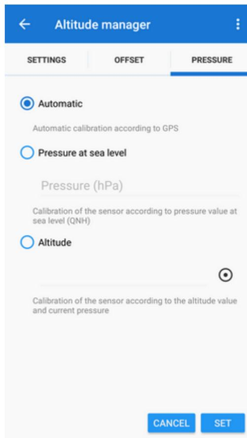
Some devices are equipped with barometric pressure sensor. Barometric sensors measure atmospheric pressure very precisely which can be used for calculating relative altitude changes. I.e. if you know certain pressure at certain altitude you can calculate altitude changes between known and current position.
