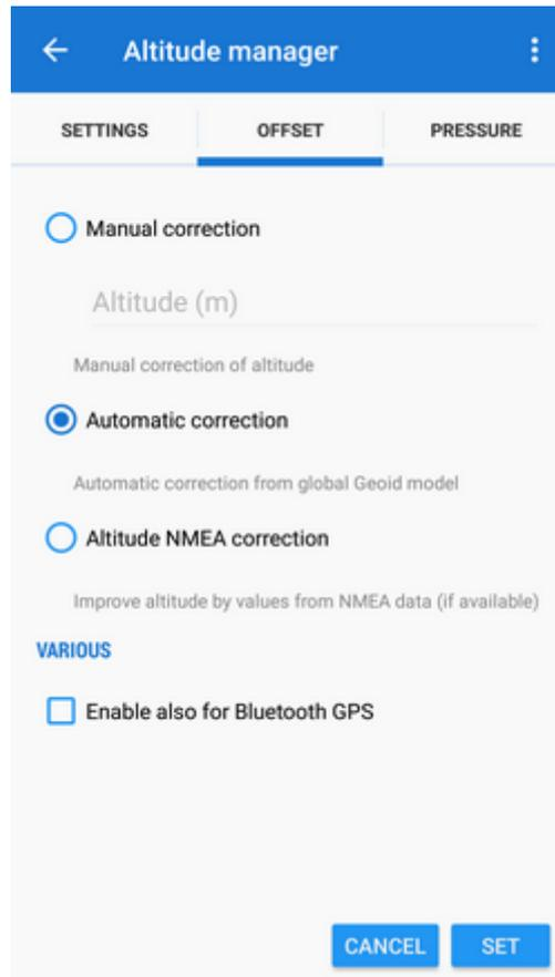
Altitude calculated by internal or external (Bluetooth) GPS unit is related to a different method of referencing the Earth surface than that used in maps. The difference between them is called **Geoid height** which is distance between [Geoid](#) and [reference elipsoid](#).
