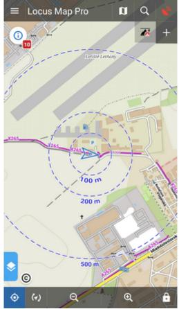
In case the GPS is fixed the circles have different color and indicate distance from the user's location.
