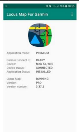
This application has to be installed on your phone to provide communication between **Locus Map** mobile outdoor navigation in your phone or tablet and Locus Map in your **Garmin** device via Bluetooth. It does not work without main Locus Map app. The application further requires **Garmin Connect Mobile** installed on your phone.
