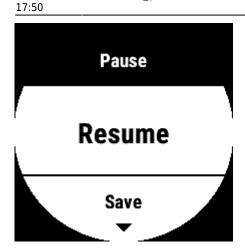
Recording can be paused or restarted by another press of the START button. If paused, the app will show a menu where user can save activity and prepare it for export to Garmin Connect. This is done automatically by Garmin device during next synchronisation with Garmin Connect Mobile or with Garmin Express desktop app. During inactive activity recording, GPS is automatically turned off to safe battery (based on app setting with 5 minutes timeout or immediately).
