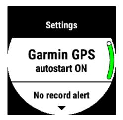
User can affect the behaviour of the application by accessing settings in the app menu. Application menu can be opened same way as watch system menus (long-press UP on non-touch watches) from any activity screen except map screens. Settings are stored in device permanent memory.
