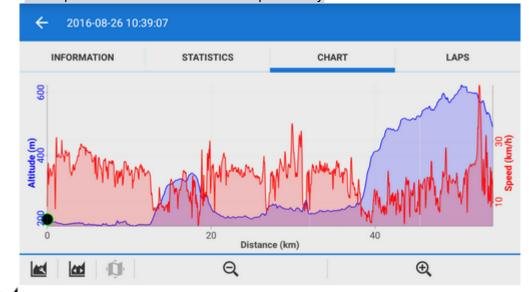
• *chart settings* - settings of the chart axes - the X axis can display distance or time, two axes Y can display altitude, gradient, speed, heart rate, cadence (in case appropriate sensors are connected and active). Navigation waypoints (if there are any) can be **hidden**.
