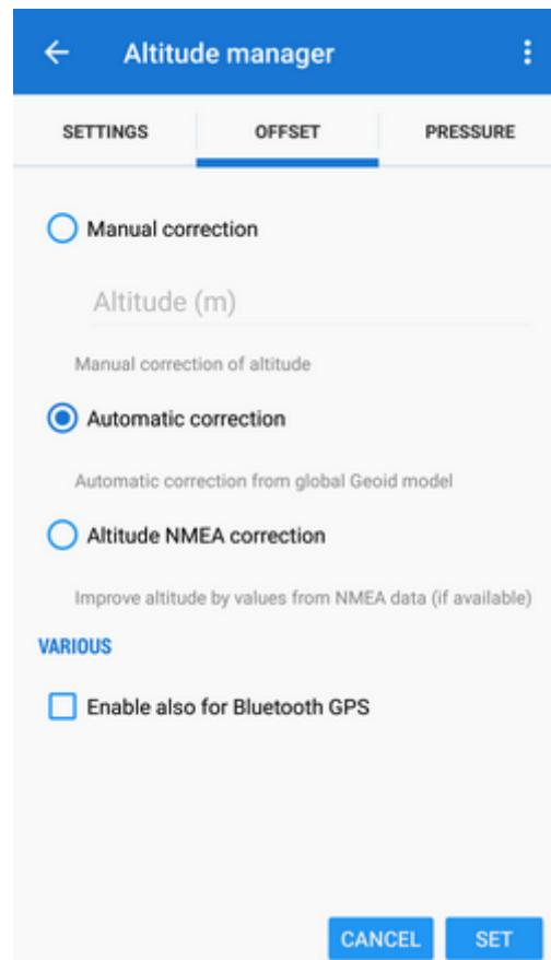
Altitude calculated by internal or external (Bluetooth) GPS unit is related to a different method of referencing the Earth surface than that used in maps. The difference between them is called **Geoid height** which is distance between **Geoid** and **reference ellipsoid**.
